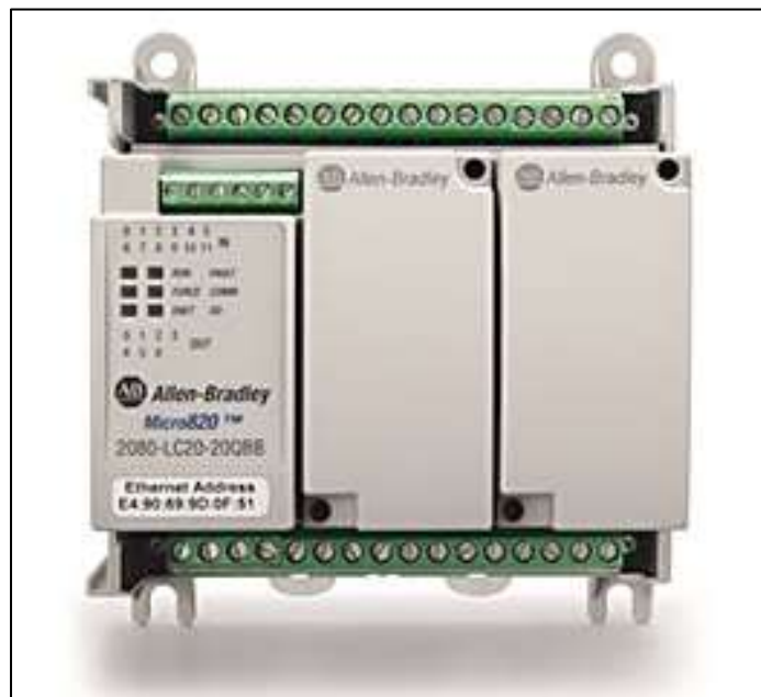
Figura 31: PLC Allen Bradley.
