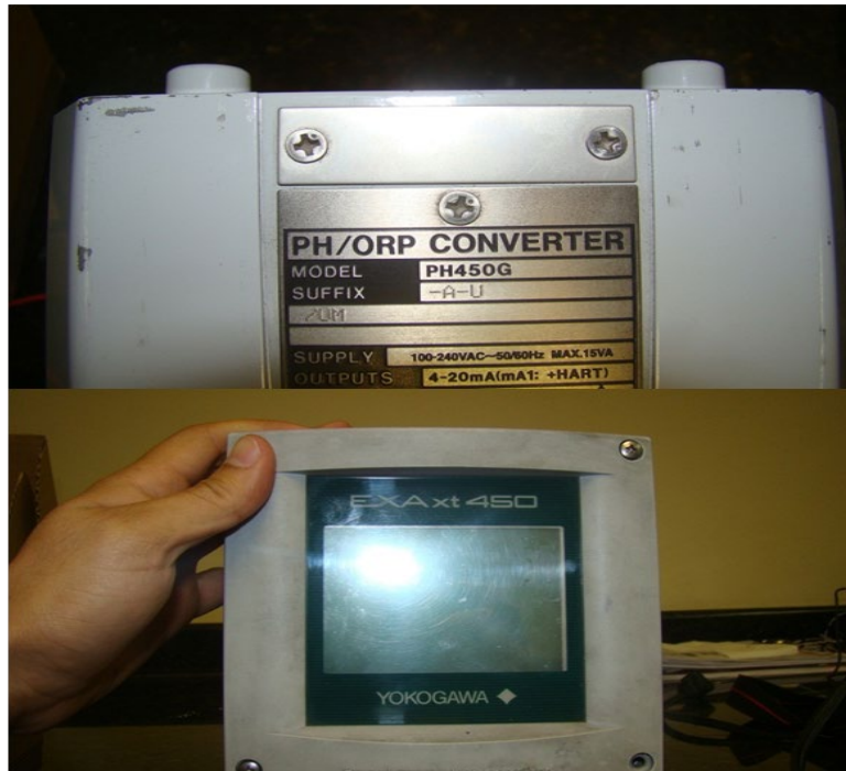
Figura 6. Transmisor Yokogawa de pH EXA xt 450
