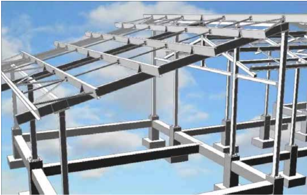
Figura 25 Pórtico Estructural https://www.youtube.com/watch?v=hajiP9c0zJ
