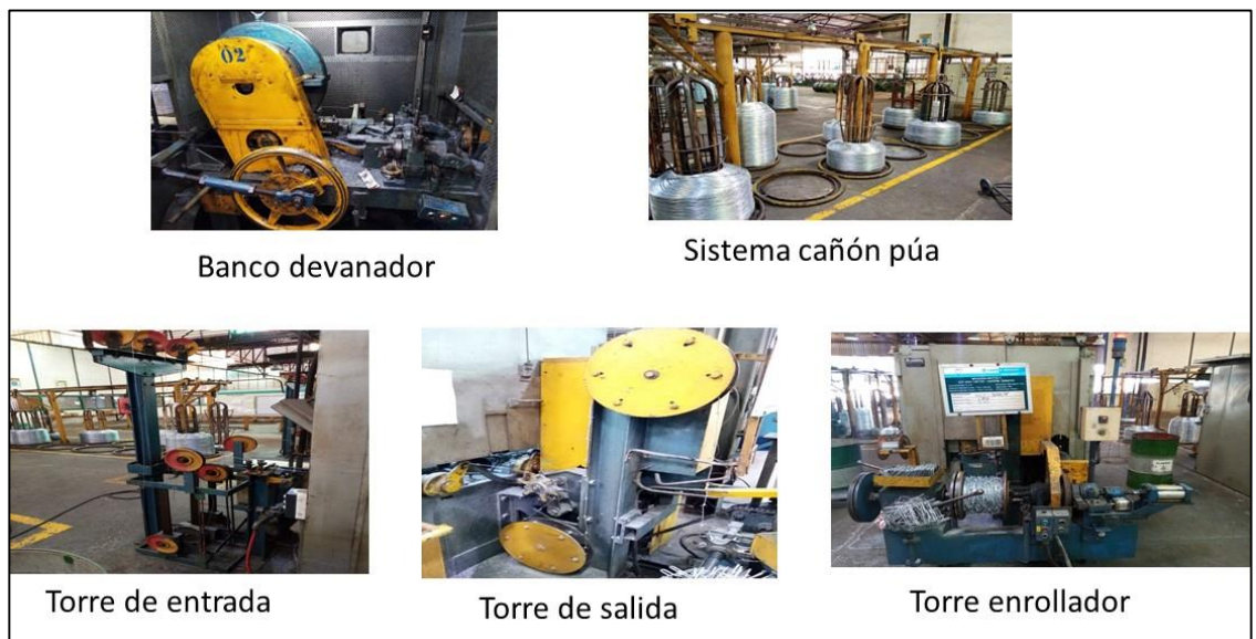
Figura 13: Partes de maquina motto
