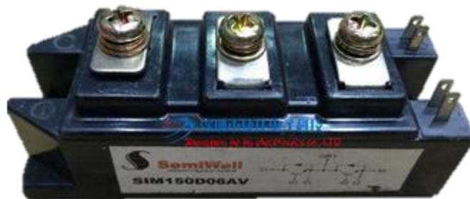
Figura 18. SemiWell half bridge IGBT Module (SIM150D06AV1) Fuente: https://www.alldatasheet.com/view.jsp?Searchword=SIM150D06AV1
