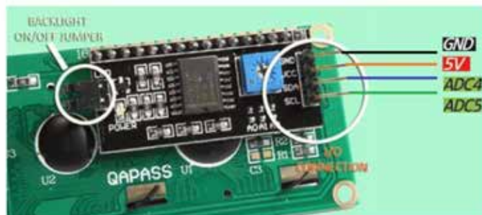
LCD display to Arduino wiring.
