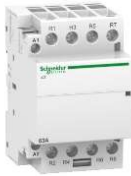
Figura 19. Contactor Schneider Electric Acti 9 iCT de 4 polos, 4 NA, 25 A, bobina 230 V ac, 1,6 W
