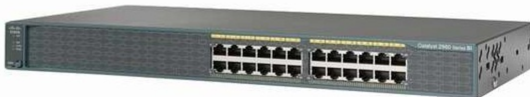
Figura 16: Switch Cisco Catalyst 2960
