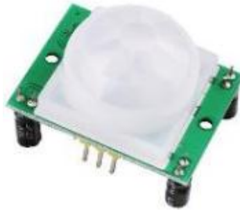
Figura 15: Sensor PIR HC-SR501
