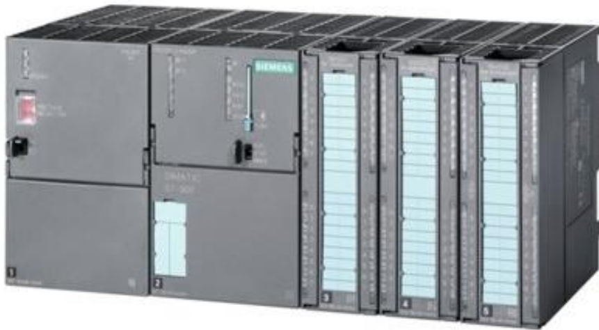
Figura 14. PLC Simatic S7-300.
