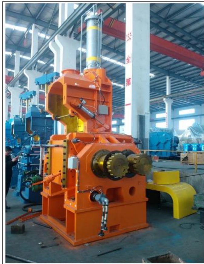
Figura N°9: Nuevo banbury sugerido a instalar Fuente: Connecting buyers with Chinese Suppliers
