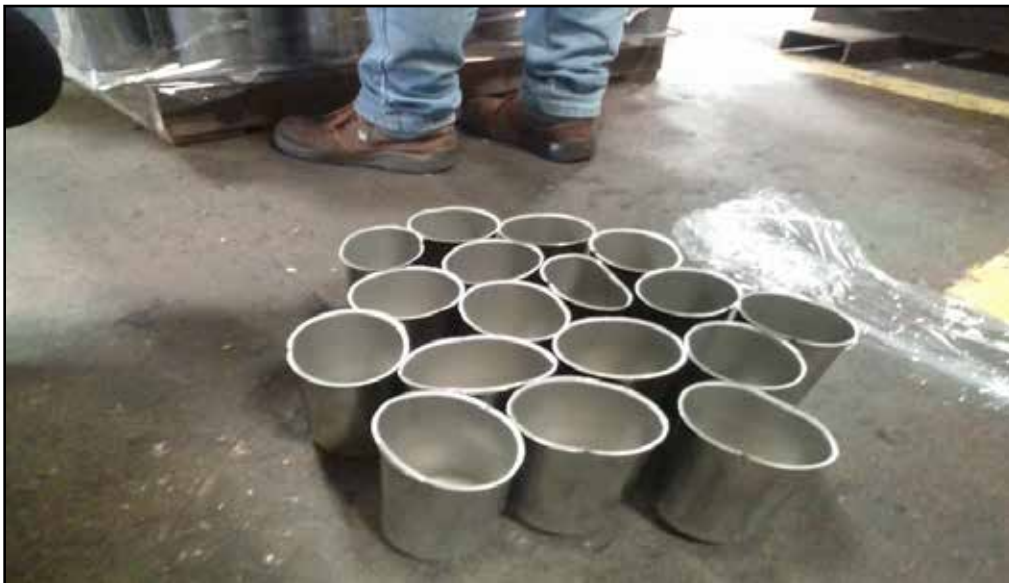
Figura 18: Vaso 47-71394 deformado . Mann+Hummel Filtration Technology Venezuela C.A (2018)
