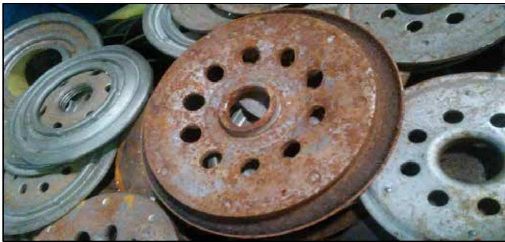
Figura 2: Tapa Cover 08-77225 oxidada parte interna. Mann+Hummel Filtration Technology Venezuela C.A (2018).
