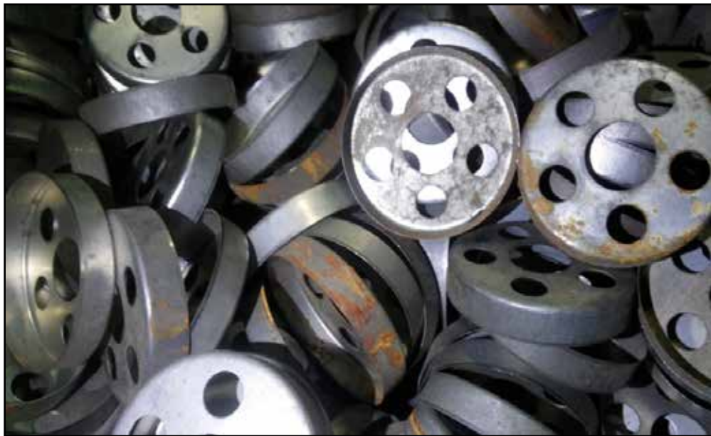
Figura 16: Guía de tubo central 02-41161 oxidada. Mann+Hummel Filtration Technology Venezuela C.A (2018)
