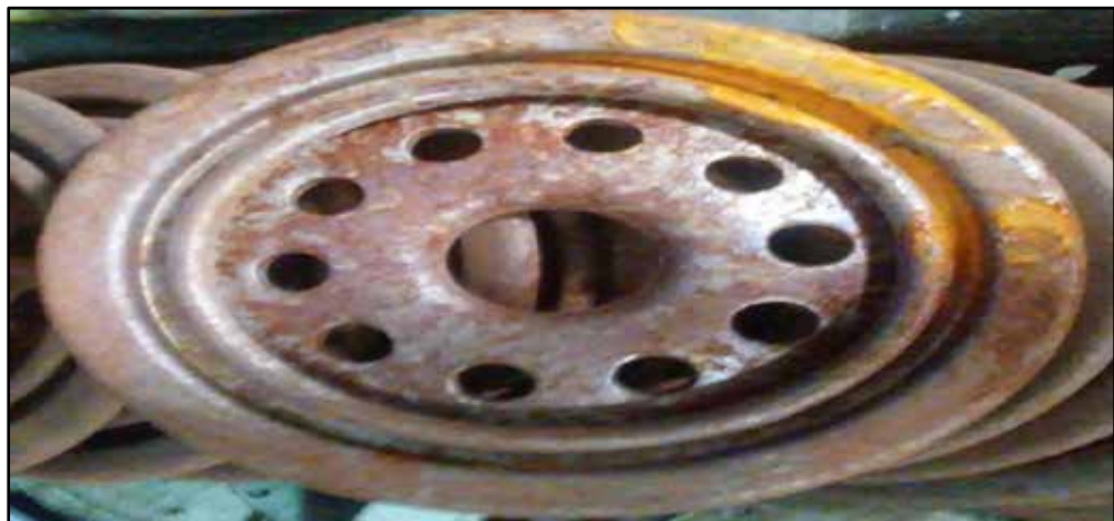
Figura 3: Tapa Cover 08-77225 oxidada parte externa. Mann+Hummel Filtration Technology Venezuela C.A (2018).
