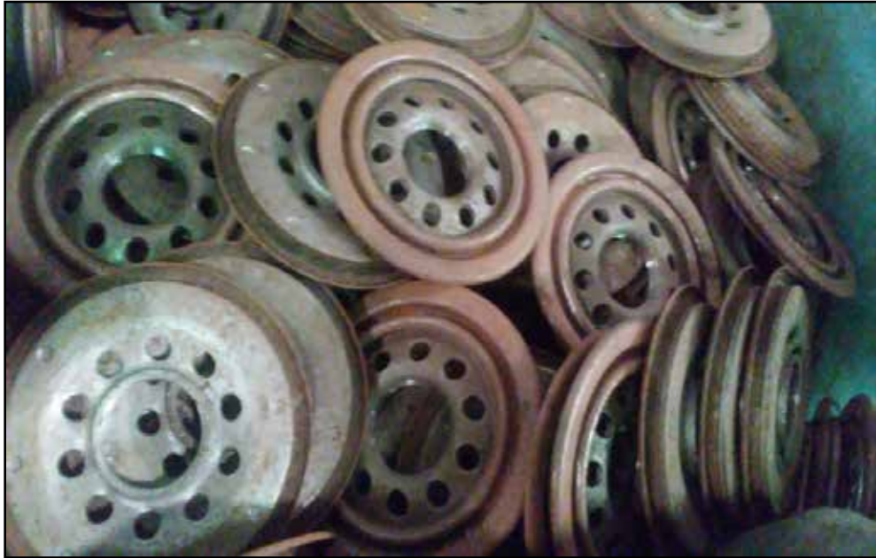
Figura 15: Tapa Cover 08-71334 oxidada. Mann+Hummel Filtration Technology Venezuela C.A (2018)
